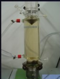
special glas reactor with cooling jacket and diffuser
